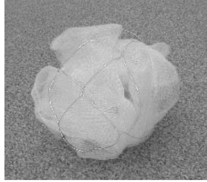
Figure 3.4: The Weedball model for the c_d measurement
