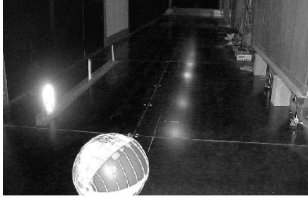
Figure 3.7: The experimental setup for the speed experiments; on the left, the 3 reflectors of the light barrier, in the foreground, a Softball model
